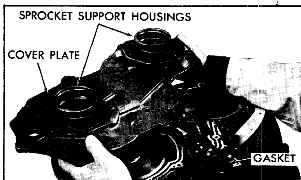
Fig. 7E-197 Installing Pump Cover Plate and Gasket
