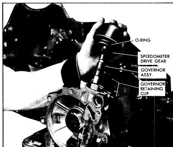
Fig. 7E-228 Installing Governor
