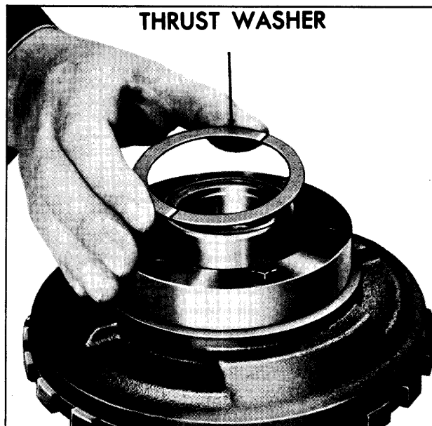
Fig. 7E-85 Removing Thrust Washer
