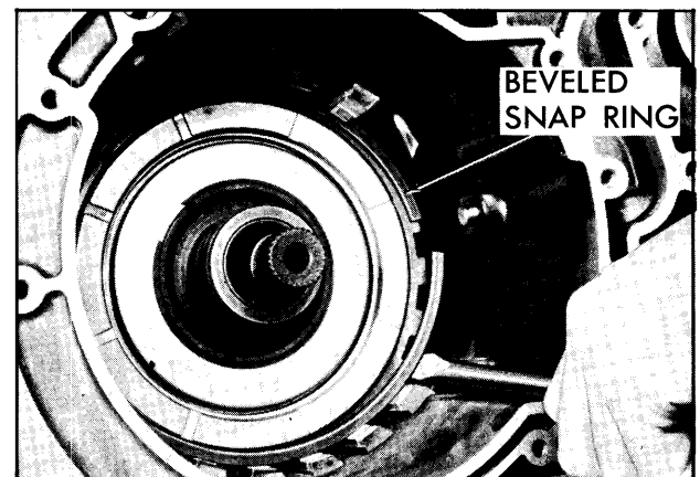
Fig. 7E-190 Installing Center Support Snap Ring
