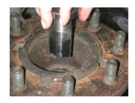
Insert the bearing guide into the top of the hub
