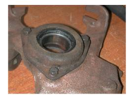
Flip the knuckle over and drop the greased "A" bearing into the knuckle
