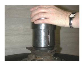
Turn the nut on threaded rod counter clockwise to remove the bearing
