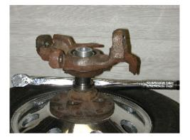
Assemble the bearing tool with the centering ring. Note that the thicker flange of the centering ring is placed at the outer edge of the split cup.
