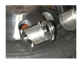
Place the greased bearing over the bearing guide.
