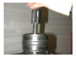
Place the split cup around bearing. Check the Problems Section of this manual if you have trouble getting the split cup to fit between the seal and the bottom of the bearing.
