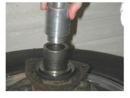
Assemble the bearing tool using the centering ring. The thicker flange of the ring is placed at the outer edge of the split cup.
