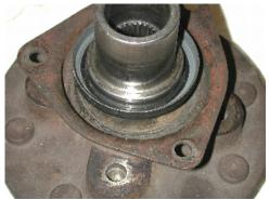
Insert the bearing guide into the top of the hub.
