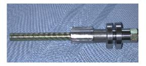
Insert the threaded rod and splined nut into top of hub as shown
