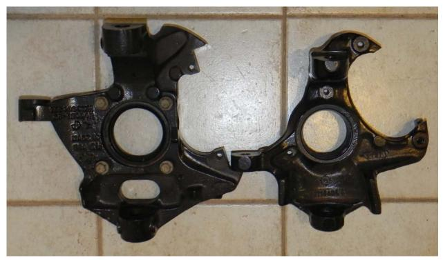
This is a comparison of the Chevy knuckle on the left and the GMC on the right. The Chevy is a taller unit, has the tie rod connection at a higher elevation and uses a similar 80MM brake unit. The Chevy has a bolt in bearing pack using four bolts while the GMC is a press fit. Pictures of this bearing pack are shown below The outside diameter on the GMC bearing is 3.05 inches and the Chevy bearing is 3.90 inches.
