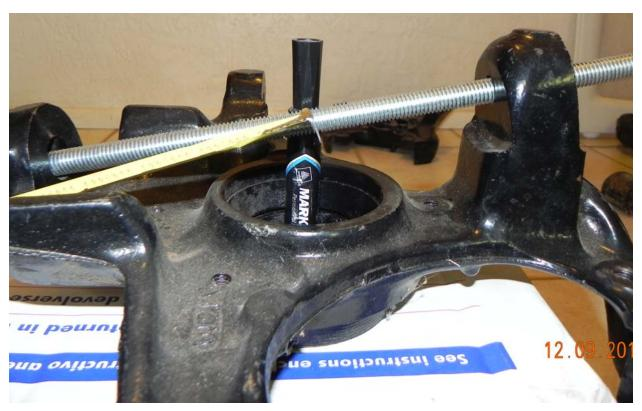
These GMC pictures show the location of the axel relative to the top of the lower ball joint mounting lug. The lower picture show about 4.875 distance from axel center to lug measured along the king pin line
