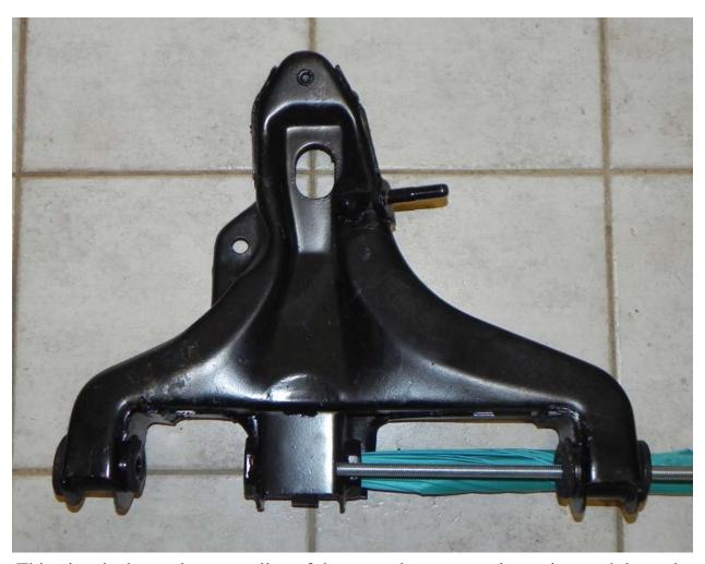
This view it shows the center line of the control arm mounting points and the teal color is the location of the torque bar also on the same centerline. Also note that the torque box is nearly aligned with the drive line
