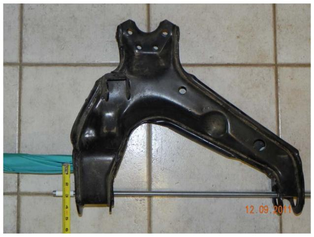
The Chevy torque bar is located about on the horizontal center line and outboard of the hinge line by 2.5 inches. The torque bar socket is 1.75 inches
