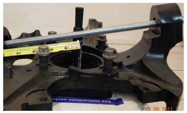
These pictures are of the Chevy axel location as measured along the king pin line. Again the distance is approximately 4.875 indicating that the axels are in the same location relative to the top of the lower ball joint lug on both knuckles.
