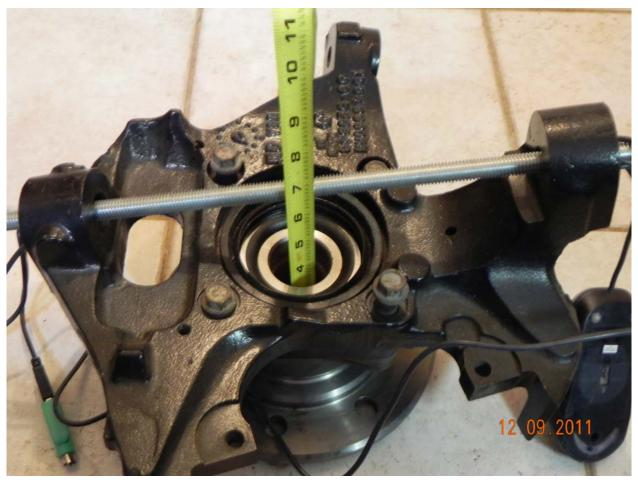
These pictures show the Chevy knuckle assembly on the floor resting on the centering flange. Measurement is taken to the king pin line for consistency from GMC to Chevy. This distance is approximately 6.5 inches and is the same for the GMC.
