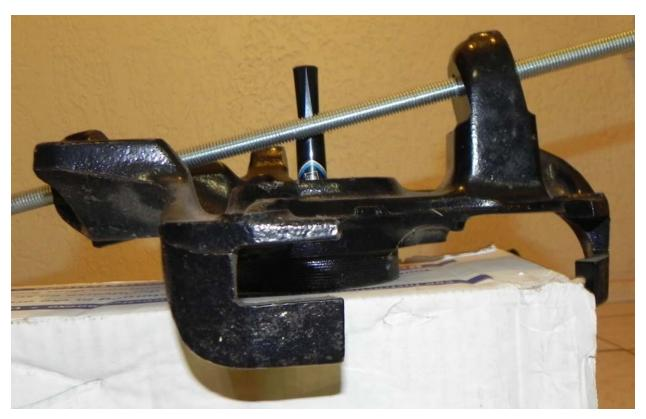
The above picture shows the GMC knuckle laying with the wheel bearing holder flat on the surface. A 1/2 inch rod is showing the king pin center line and the magic marker is centered in the bearing holder. The pictures below are showing the distance between the Lower ball joint mounting hole top surface and the upper ball joint mounting also on the upper surface. This distance is approximately 9.5 inches.
