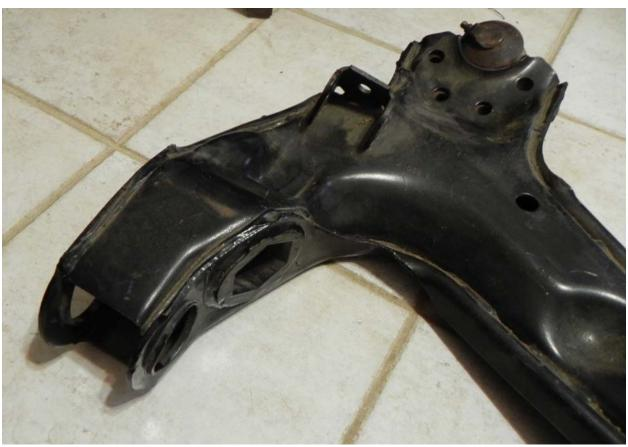
The Chevy socket is a square cut on the outboard side but is a slant cut on the inboard, The length is 3 5/8 on the short side and 4 1/2 on the long side. The GMC socket is square cut at 4 1/4 inches.
