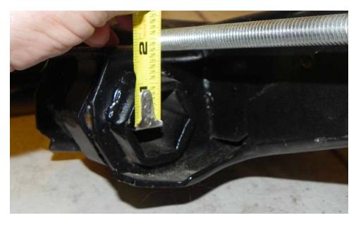
This view shows that the center of the torque box is about two inches directly below the hinge line. The GMC socket is 1.5 inches
