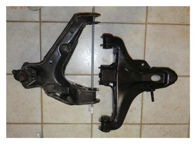
This photo shows the relative position when the drive lines are aligned. The Chevy, on the left, mountings are much more forward on the frame than the GMC. Again, see the relative length difference for the torque bar.
