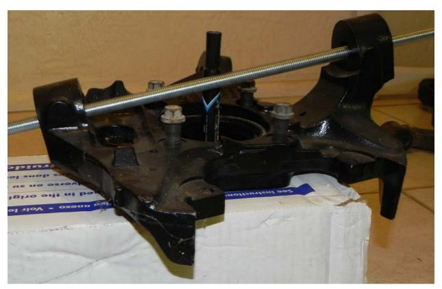
This picture shows the Chevy knuckle laying on the bearing flat surface with a rod thru the ball joint holes to show king pin angle. Also the marker is located in the center of the bearing hole. The lower picture on the left shows measuring from top to top on the ball joint mounting holes. The picture on the lower left shows a measurement of 11.5 inches. This is exactly 2.0 inches taller than the GMC knuckle.
