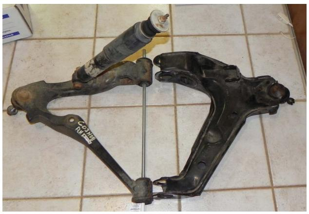
A comparison of the early design control arm from about 1988 through 2000 to the current design starting in 2001. Major difference is welded assembly to a forged steel assembly and the difference in ball joints. Early was mounted with four rivets and late model is press fit.
