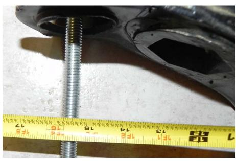
The Chevy distance from the center of the top of the ball joint to the center line of the mounting hinge is approximately 15.5 inches.
