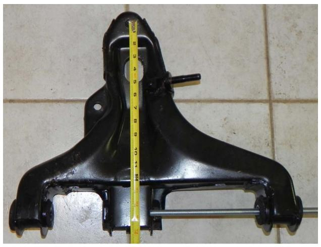
On the GMC the distance from the top of the ball joint to the hinge line is about 14.5 inches
