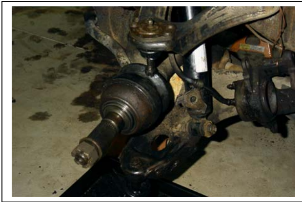
Fig. 13. This picture illustrates both the upper and lower control arms as well as the drive shaft with outer CV joint. Hub and knuckle are removed in this view. Note castle nut in place on the axle shaft.
