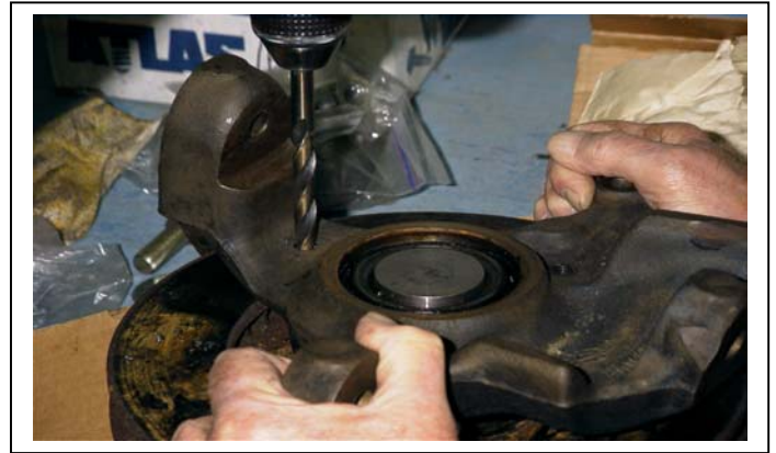
Fig. 6 This photo illustrates drill enlargement on the back side of the knuckle of the outer grease seal retainer plate bolt holes when needed, prior to chasing/tapping.
