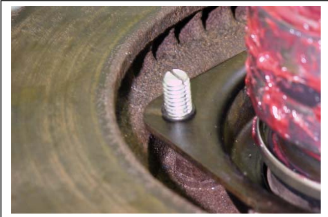
Fig. 18 This view illustrates slot for screwdriver cut across end of outer seal retainer plate bolts. Note “O” ring retaining bolt in seal retainer plate.
