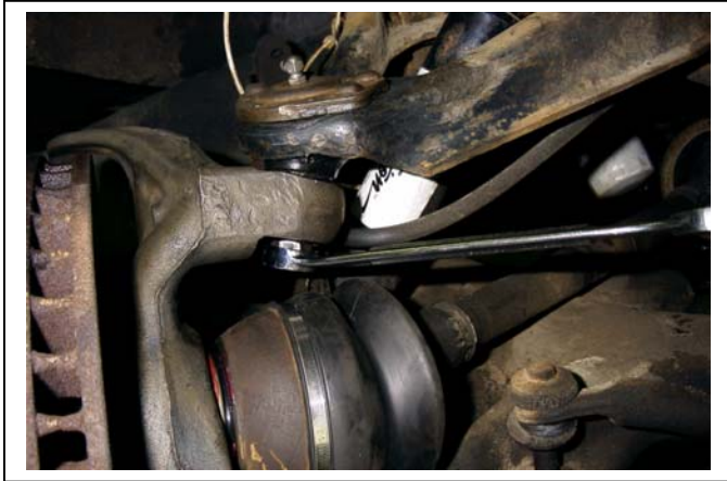
Fig. 28. Upper ball joint nut being tightened in place.
