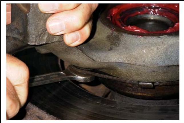
Fig. 5. Outer grease seal retainer bolts being loosened.
