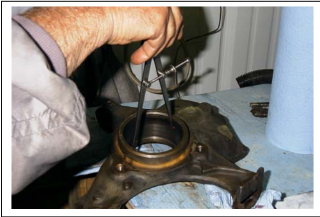
Fig. 16. Measuring bore of knuckle with caliper.
