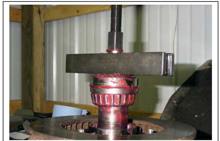
Fig. 22. Bearings stacked on top of hub shaft. Note OTC cross block bar and pressing/forcing screw in place on the shaft. HOWEVER, THE ABOVE PICTURE ILLUSTRATES THE WRONG SEQUENCE OF BEARING ASSEMBLY.
