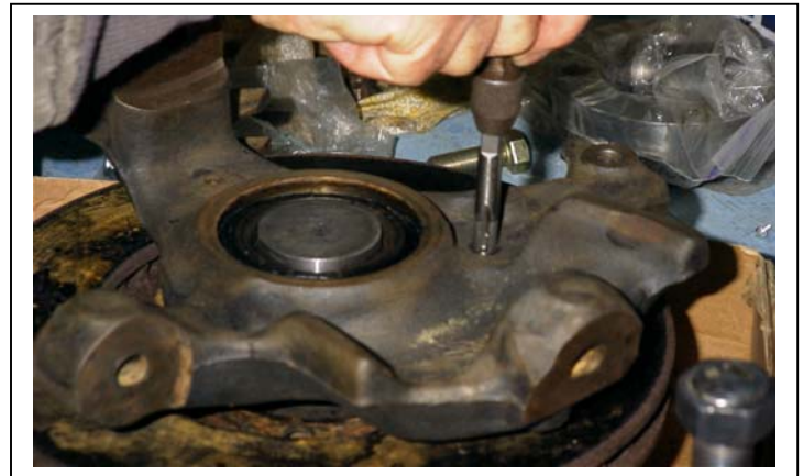
Fig. 7. Chasing/tapping outer grease seal retainer plate bolt hole threads in the knuckle.
