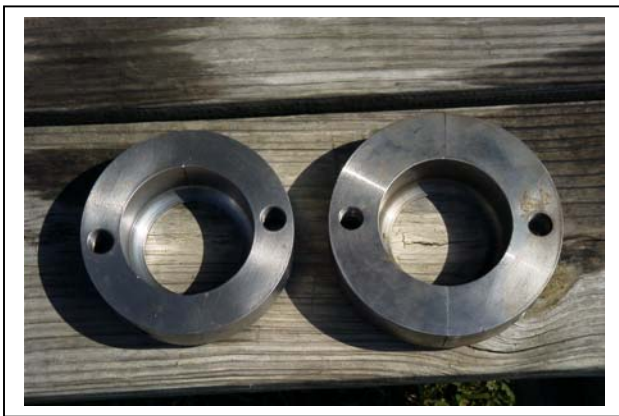
Fig. 11. This view shows the two different diametered Warner bearing puller tool bearing clamps.
