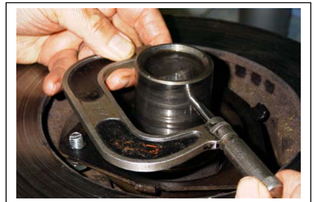
Fig. 15. Caliper being used to measure hub shaft dimension.
