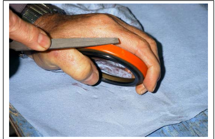
Fig. 28. Using a file to chamfer metal edge of inner seal .
