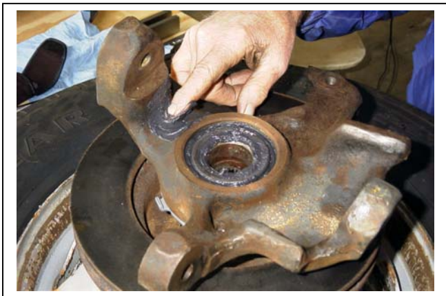
Fig. 27. Packing bolt holes with grease.
