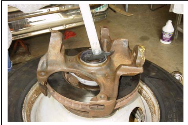
Fig. 8. Inner grease seal removal.
