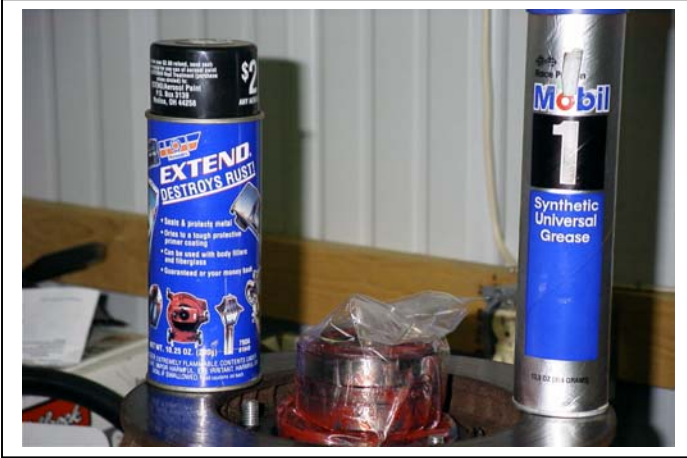
Fig. 1. Permatex Extend aerosol spray can, shown on the left, used for corrosion control (it encapsulates any remaining rust and dries black in color) and Mobil 1 tube of synthetic grease, shown on the right, used to pack bearings. Packed bearing set, shown in the center of the picture, is protected by a plastic “baggie”.
