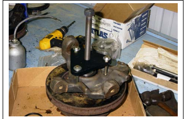
Fig. 10. Warner bearing puller tool knuckle puller plate bolted in place shown with puller screw in place.
