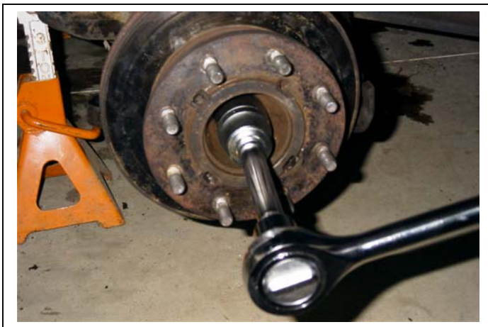
Fig. 30. Axle nut being tightened (turn in clockwise direction for both sides).
