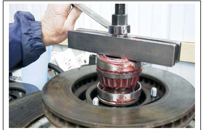
Fig. 24. Press bearings onto hub shaft by turning nut on the pressing screw with a wrench. HOWEVER, ONCE AGAIN THE ABOVE PICTURE ILLUSTRATES THE WRONG SEQUENCE OF BEARING ASSEMBLY. Anytime the bearing race drops down, as shown above, THAT IS INCORRECT assembly. In this example, reverse lower bearing and reassemble stack in the proper sequence.
