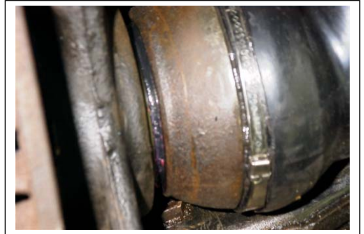
Fig. 31. Tightening axle nut draws the outer CV joint, seen on the right side above, in close proximity to back side of the knuckle, on the left side, and in the process seats (remember in step 12 above the grease seal was set ~ 1/8 th inch above the knuckle) the inner grease seal lips.
