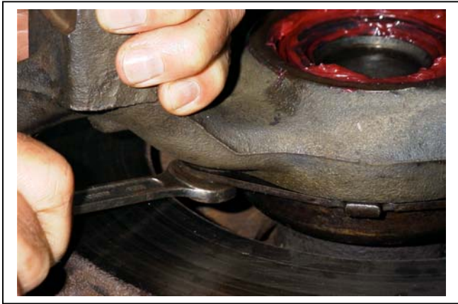
Fig. 26. Outer grease seal retainer bolt being tightened.
