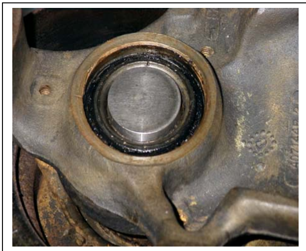
Fig. 9. Circular Warner bearing puller tool plate (i. e. aka “puck”) placed over end of hub shaft. Puller screw point bears on this plate when pulling the knuckle off the hub.
