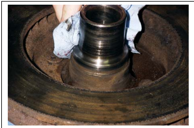
Fig. 14. Cleaning hub shaft.
