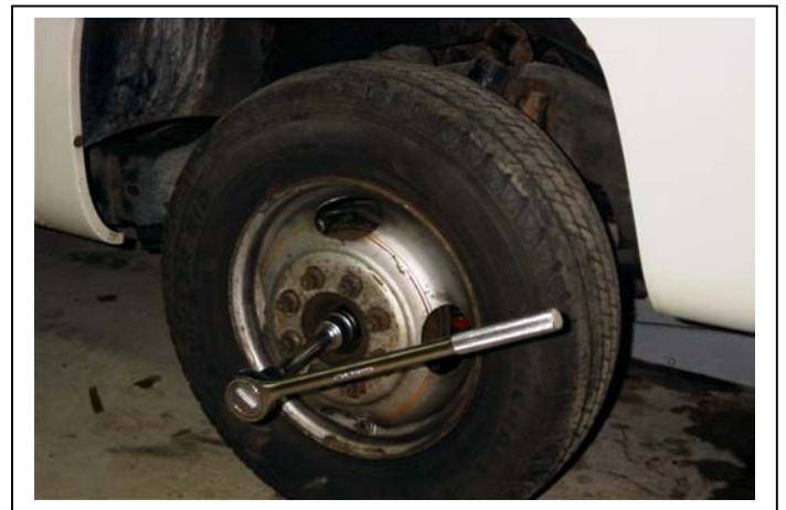
Fig. 2. Note 3/4” drive ratchet with extension and 1-1/2”socket over drive axle nut. Turn wrench in conventional counterclockwise direction to loosen nut, both driver and passenger sides.
